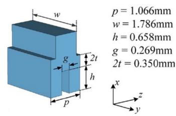
Top: single-element 3-D schematic of the SWS with geometric parameters (Lai et. Al)
