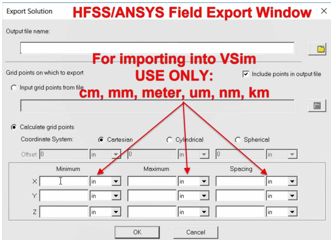
Fig. 5.11: Grid settings (size and units) for exporting a field file from HFSS/ANSYS. For converting to VSIm field files, the units that should be used are cm, mm, meter, un, nm, and km. IMPORTANT: these grid settings must be consistent with the Grid settings in the Grids element tree in the VSIm setup window.
